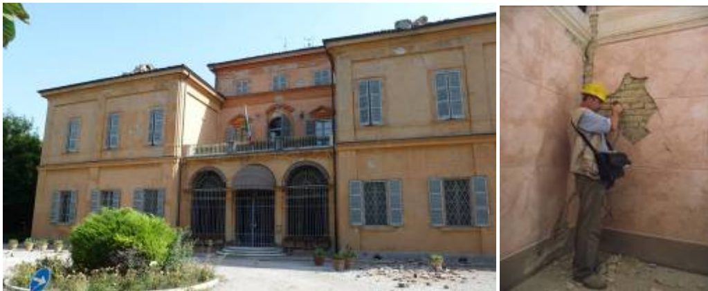
Casa di cura, Cantone street (view and PNT-G tests on mortar joints)
